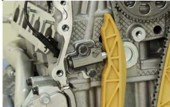
**Figure 11:** 2.4L Timing Chain Tensioner
