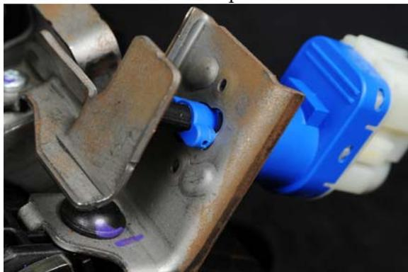
*Figure 23: Brake Pedal Switch Comes in Contact with Bracket During Installation*
