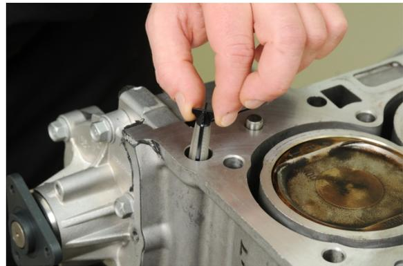
**Figure 8:** Filter Screen Installed in Cylinder Block
