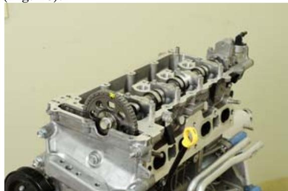
**Figure 13:** MultiAir Brick Removed
