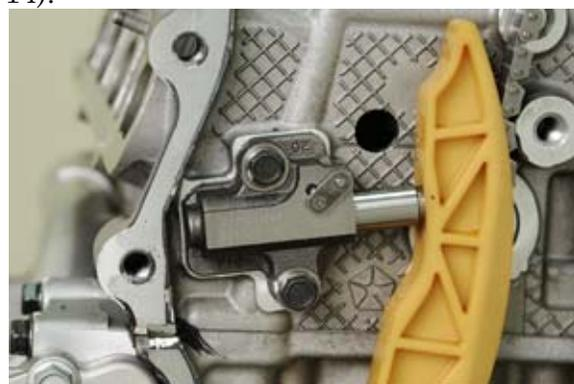
**Figure 14:** Timing Chain Tensioner Extended
