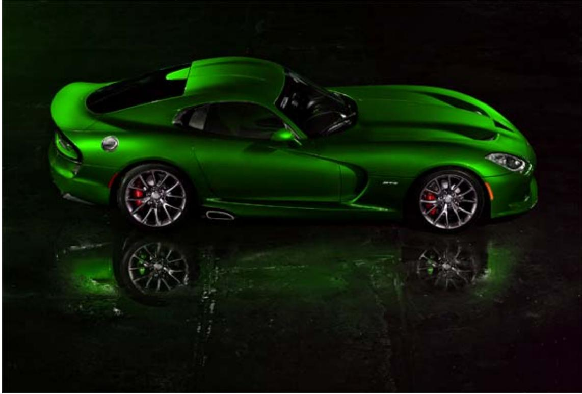
**Figure 26:** Carbon fiber hood, roof, and deck lid shave weight
