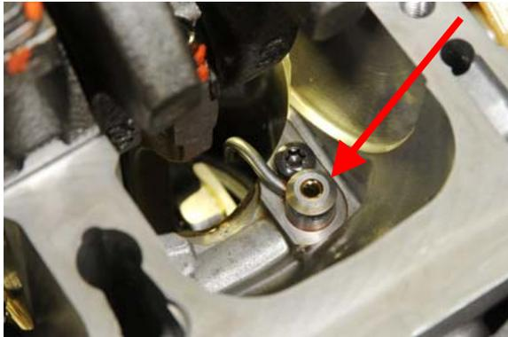
**Figure 6:** Piston Cooling Jets
