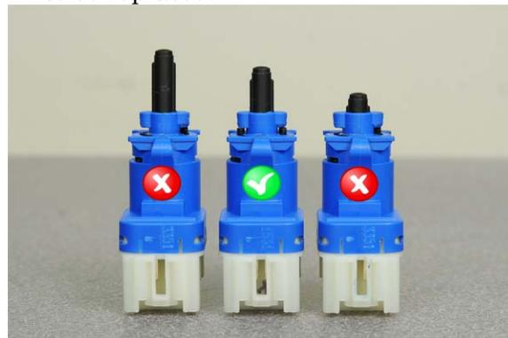
**Figure 22:** *Undamaged Plunger Compared to Damaged Plungers*
