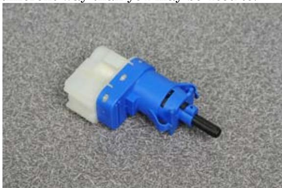
**Figure 21:** *New Brake Pedal Position Switch*
