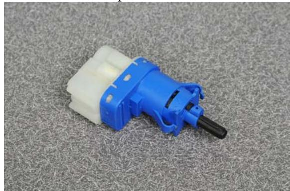
**Figure 3:** Dart Brake Pedal Switch
