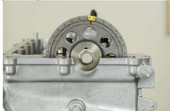
**Figure 20:** Timing Chain Access Cut-out
