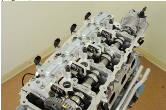
**Figure 10:** 2.4L MultiAir Valvetrain
